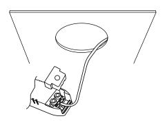
4.Make sure the downlight ⊠xed tightly in ceiling, turn on the power.
