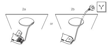
4. Make sure the downlight fixed tightly in ceiling, turn on the power.
